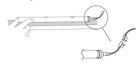
\*If longer cable is required, order battery extension cable to increase cable length to 48" or 96"
